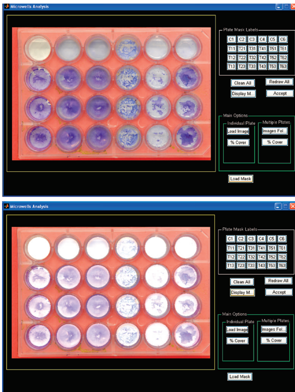
Figure 4. Coating array plate image loaded into the graphical user interface (top). Mask applied to the plate image (bottom). White regions of the mask show the precise area used to calculate percent surface coverage for each well of the coating array plate.
